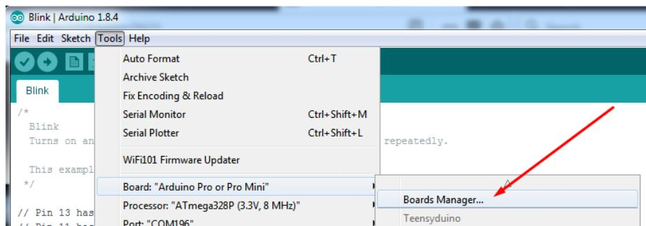
Once the Board Manager opens, click on the category drop down menu on the top left hand side of the window and select **Contributed**. You will then be able to select and install the boards supplied by the URLs added to the preferences. In the example below, we are installing support for *Adafruit AVR Boards*, but the same applies to all boards installed with the Board Manager.
