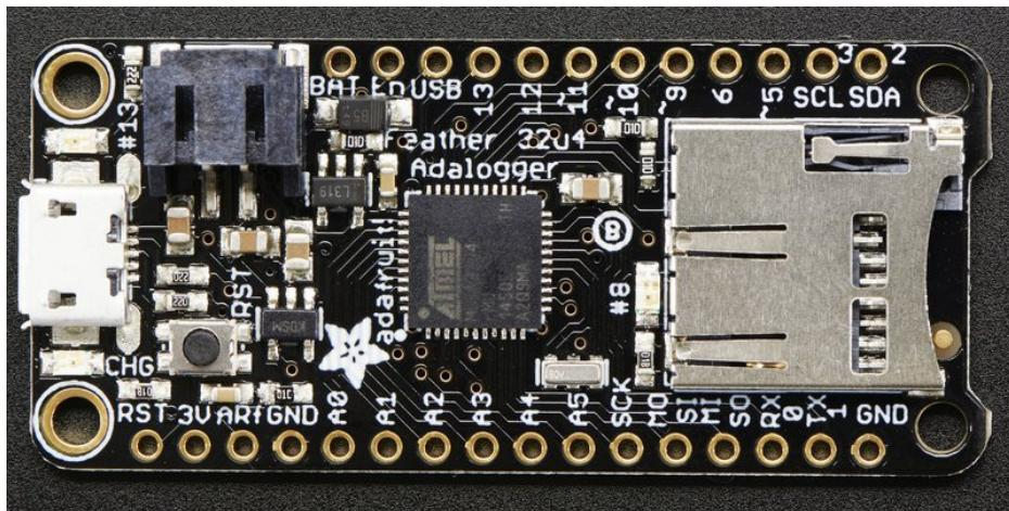
At the Feather 32u4's heart is an ATmega32u4 clocked at 8 MHz and at 3.3V logic, a chip setup we've had tons of experience with as [it's the same as the Flora](#) (<https://adafru.it/dVl>). This chip has 32K of flash and 2K of RAM, with built in USB so not only does it have a USB-to-Serial program & debug capability built in with no need for an FTDI-like chip, it can also act like a mouse, keyboard, USB MIDI device, etc.
