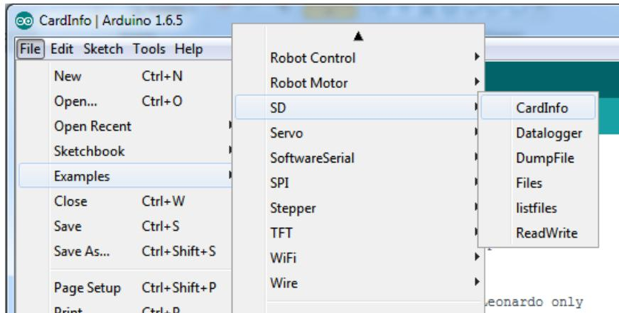
Luckily many of the default examples already have **chipSelect = 4** so you can just upload immediately. For other sketches, do check to make sure that CS is set to 4! The SD card uses hardware SPI for the remaining pins.
