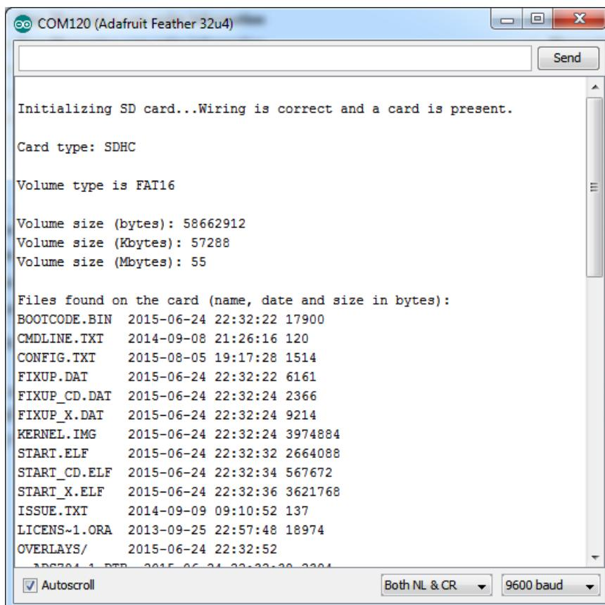
Once you have that working, check out the other examples, such the **Datalogger** example (saving analog data to SD card) and **Dumpfile** example (reading back data from an SD card)
