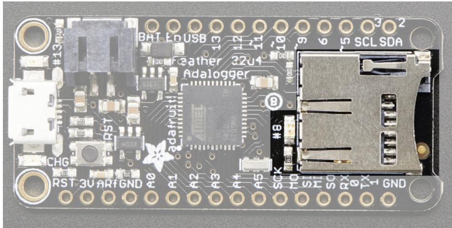
Since not all pins can be brought out to breakouts, due to the small size of the Feather, we use these to control the SD card!
