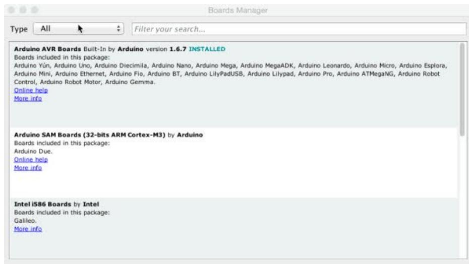
Next, quit and reopen the Arduino IDE to ensure that all of the boards are properly installed. You should now be able to select and upload to the new boards listed in the **Tools->Board** menu.
